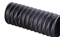
NL6114 PA-EX Self-Extinguishing 2-Ply Polyester Acrylic Urethane Blend Coating - used for pneumatic blower of light materials, particulate removal, ducting (2"-24"ID)
