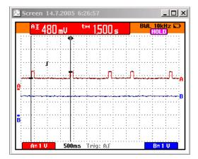
A=Pin 2 voltage Pulse ratio approx. 10 %, pause current 40 % and cycle time 1,5 s (0,7 Hz)
