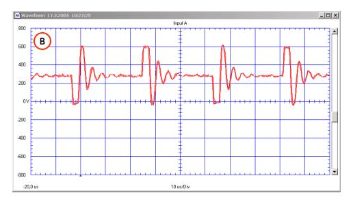
Voltage over the lower IGBT with minimum power (2800/3500). Inverter operating frequency approx. 19 kHz (measuring point B).
