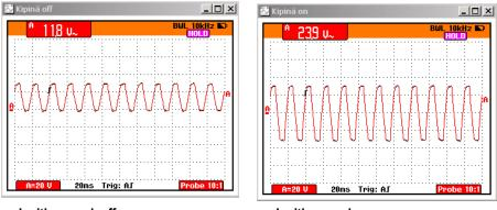
Measured between connectors X5/1 and X5/2
