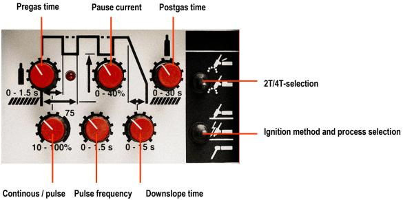
Continous / pulse Pulse frequency Downslope ti welding selection, pulse ratio adjustment
