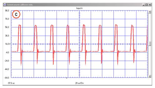
Voltage over the secondary diodes with minimum power(2800/3500). Frequency is approx. 38 kHz (measuring point C).
