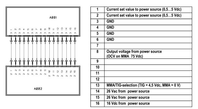
The control card A002 uses the 24 Vac to control the solenoid valve and spark ignition, and transforms the + 16 V voltage to + 5 V for control electronics.
