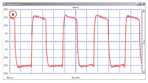
IGBT gate pulse with maximum power (2800/3500). Inverter operating frequency approx. 19 kHz (measuring point A).
