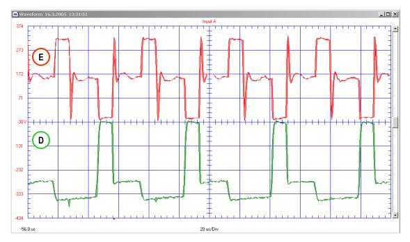
Lower IGBT control (Gate pulse; measuring point D / Voltage over the lower IGBT; measuring point E).
