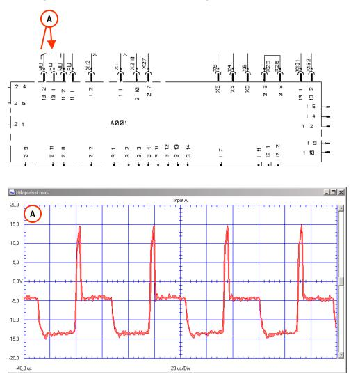
IGBT gate pulse with minimum power (2800/3500). Inverter operating frequency approx. 19 kHz (measuring point A).
