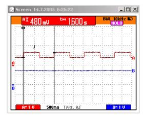
A=Pin 2 voltage Pulse ratio approx. 50 %, pause current 40 % and cycle time 1,5 s (0,7 Hz)
