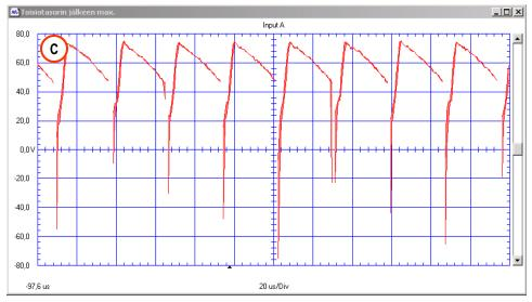
Voltage over the secondary diodes with maximum power (2800/3500). Frequency approx. 38 kHz (measuring point C).
