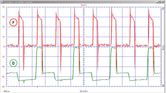
Voltage after the secondary diodes (measuring point F) and lower IGBT gate pulse (measuring point D).
