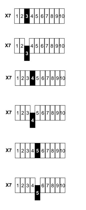
Gas/Water cooled gun selection switch bypassing (always in water position).
