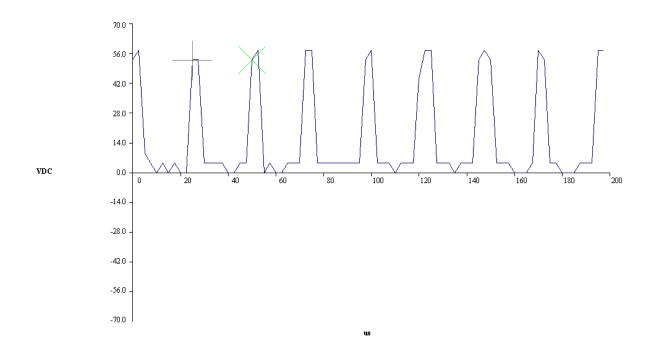
Wire feed motor control Wire feed speed: 8 m/min U<sub>peak</sub>: 57 V U<sub>average</sub>: 11,22 V Frequency: approx. 40 000 Hz
