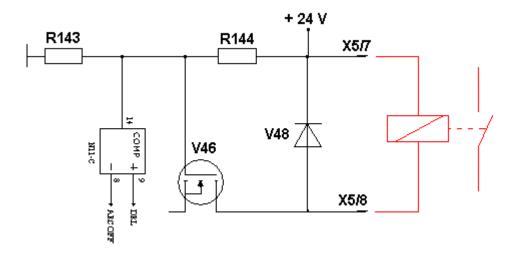
Arc on/off-signal can be used to control for example mechanization devices ON/OFF.
