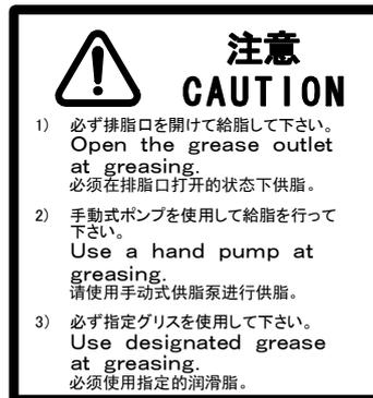
Fig. 8 (a) Greasing and degreasing label
