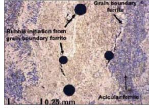
Hydrogen bubble initiation and propagation from  $\boldsymbol{\alpha}$  grain boundary.
