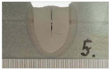
Weld depth to width ratio > 1 and relatively large amount of impurities in base material (S, P, Nb).
