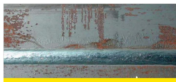
OK Flux 10.88 on rusty plate with mill scale. Porosity-free, shiny weld appearance. Clean weld with no indication of slag residues adhered onto the bead or along the toes of the weld.
