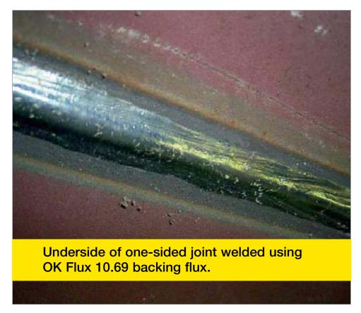
An agglomerated, basic flux specifically designed as a backing flux for one-sided submerged arc welding.
