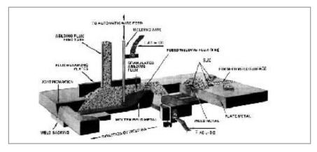
current flows between the electrode and the work.
