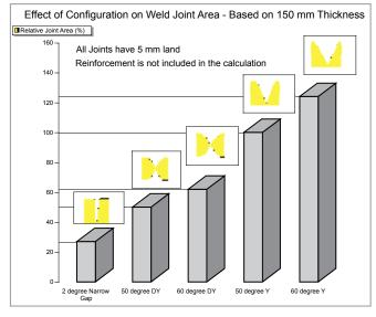
In 150 mm material thickness, 5 mm land - reinforcement not included.
