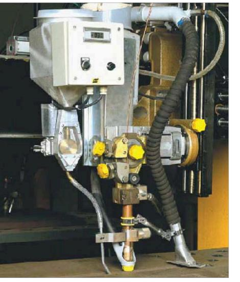
Flux 10.62/OK Autrod 12.32 is the most common.
