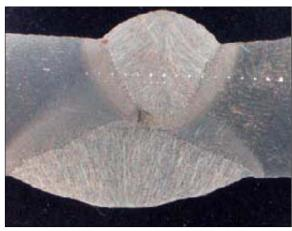
Insufficient penetration and excessive reinforcement; also misaligned.
