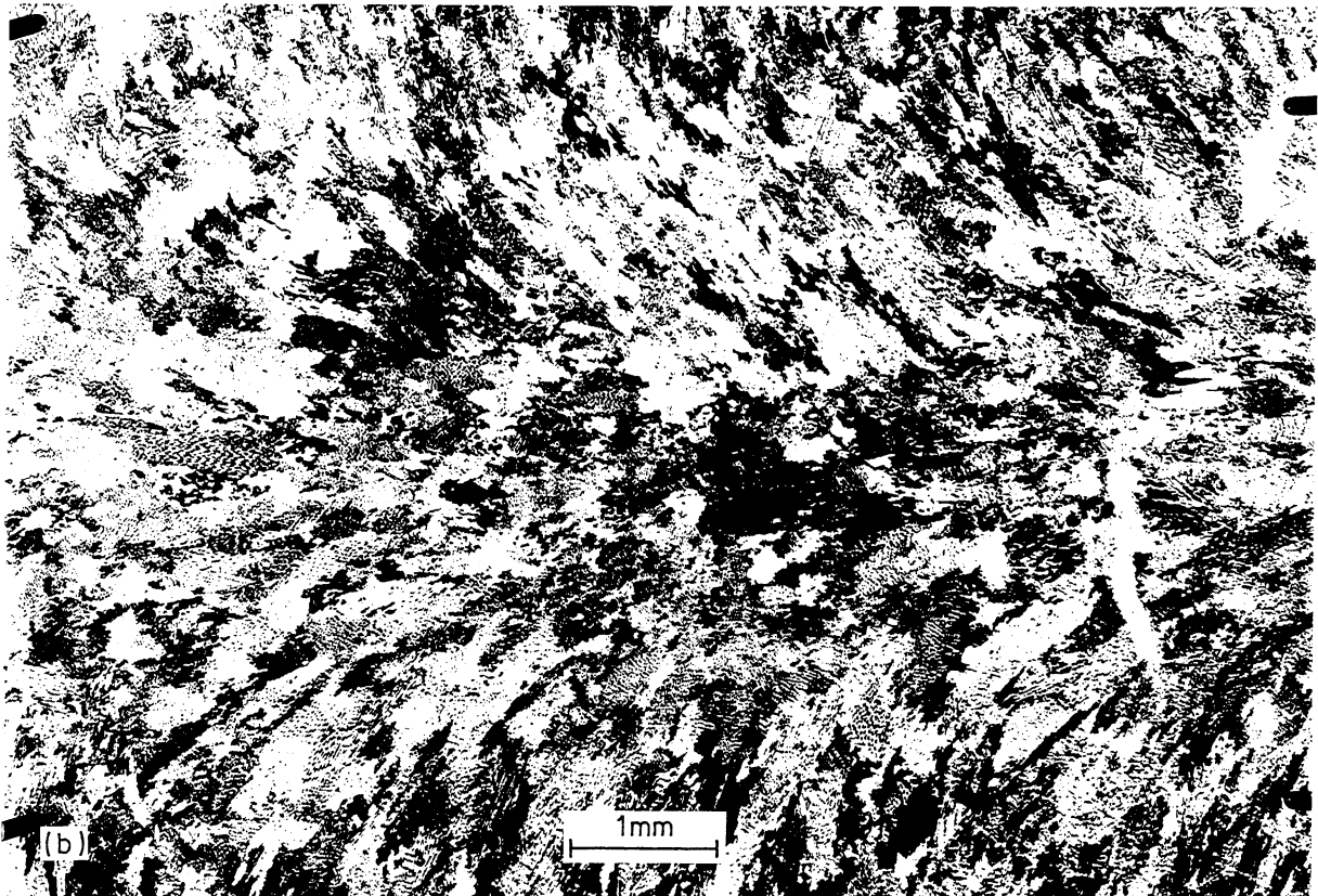
6 Grain growth in TIG welded AISI 321 stainless steel with modulated slope-out: a) Natural columnar formation without modulation; b) Modulation at 10 Hz.
