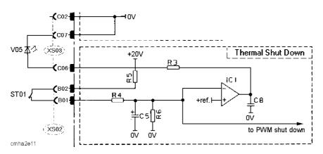
This circuit interrupts the gate pulses from the pulse width modulator if the machine is overloaded. When it has not operated due to high temperature, the thermal overload cutout normally short-circuits inputs B01 and B02. If the cutout contact opens, IC1 lights LED V05 and the pulse width modulator (8) blocks the gate pulses. See also ST01 in the component description.
