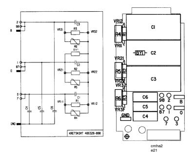
Circuit diagram and component positions circuit board AP05
