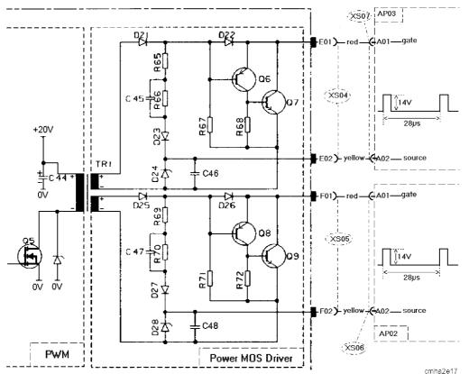
The driver stage for the MOSFET transistors provides control pulses to the gate-source of the power transistors. There is a separate output for each switching unit.
