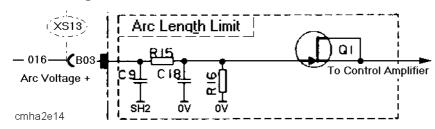
This circuit, which restrict the arc voltage and open-circuit voltage, assists in limiting the arc length when welding in the 20 - 50 A current range.
