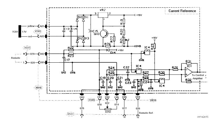
This circuit supplies a signal voltage to the current setting potentiometer and remote control unit. It also modifies the current reference signal to a suitable level for the control amplifier (7).
