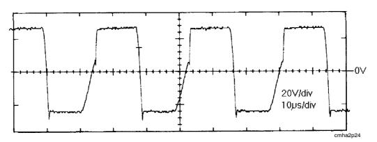
Primary voltage at TC02 for 30 V across the buffer capacitor
