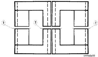
Airgap (t) in the transformer core
