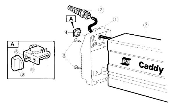
Removal of the rear panel and casing
