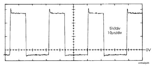
Gate pulses as measured across the dummy gate load on circuit board AP01 between connections F01 and F02.
