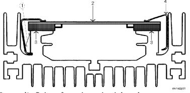
Removal/refitting of transistor circuit board
