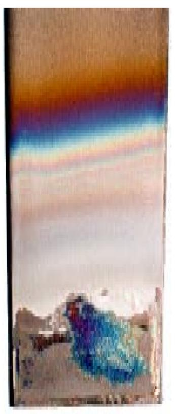
A pieceof titanium sheet 10mm wide, the lower edge of which has been heated (in air) showing the effect of progressive oxidation and increasing oxide thickness.
