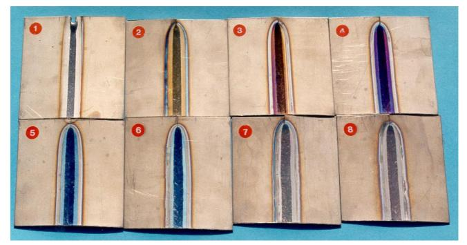
TIG welds in commercially pure titanium sheet made with successively greater air contamination of the shielding gas.
