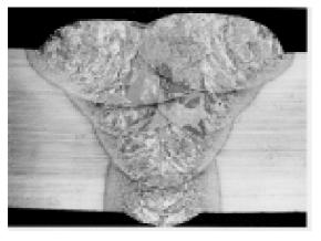
Properties of a keyhole plasma arc weld in 14mm (.55")thick Ti-6AI-4V
