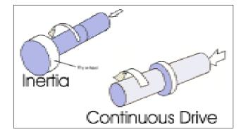
Schematic diagrams of the two rotary friction welding variants
