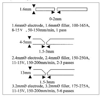
Manual TIG welding of a titanium vessel (Bunting Titanium)
