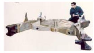
Titanium alloy (grade 5) fabricated structure for high specification military application
